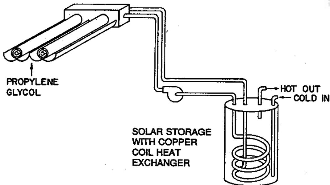
**Figure A6-2. United States Dream System for Freezing Climates.**
