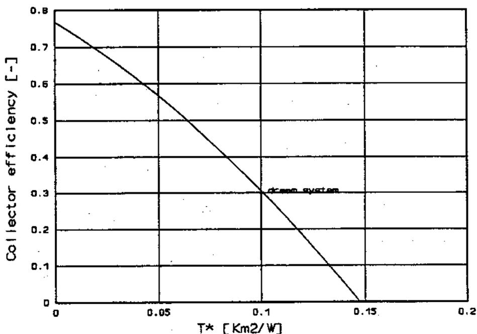
**Figure A4-4. The Netherlands Dream System Collector Efficiency Curve.**
