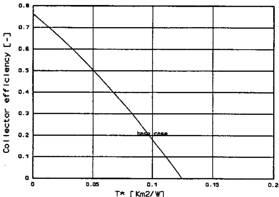
**Figure A4-2. Base Case System Collector Efficiency Curve.**
